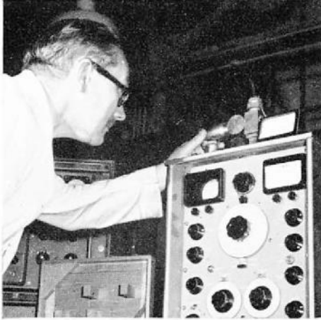
LEFT: An R.F. Test Set TF 890A going through Final Test. Dick Mapplebeck checks the frequency of the internal wavemeter against a known standard. RIGHT: Walter Elkin, Design, checks the transmission field strength of the F.M. transmitter at Wrotham by means of the TF 995A|A F.M./A.M. Signal Generator and the TF 801A|A Signal Generator
