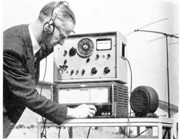
LEFT: An R.F. Test Set TF 890A going through Final Test. Dick Mapplebeck checks the frequency of the internal wavemeter against a known standard. RIGHT: Walter Elkin, Design, checks the transmission field strength of the F.M. transmitter at Wrotham by means of the TF 995A|A F.M./A.M. Signal Generator and the TF 801A|A Signal Generator
