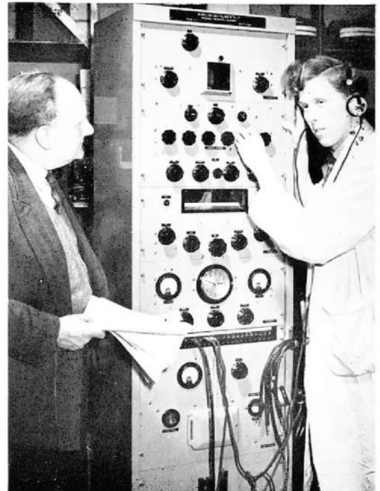
ABOVE: Dennis Brown, Calibration, standardising a TF 1066 F.M./A.M. Signal Generator, one of the new M.I. instruments. The M.I. test gear he is using comprises a Decade Attenuator, a Beat Frequency Oscillator, and two types of Crystal Calibrators
