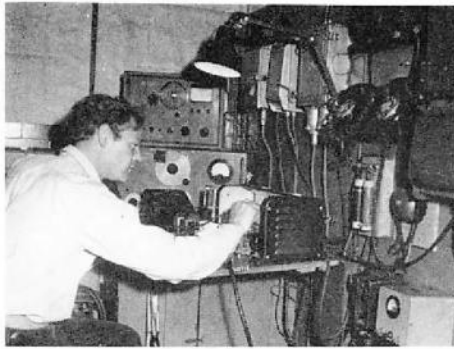
LEFT: For the maintenance of VHF equipment, a wide variety of M.I. test equipment is available. The picture shows Standard Signal Generator TF 144G and F.M./A.M. Signal Generator TF 995A being used in the repair of a mobile unit, one of many employed by a South Wales steel plant. RIGHT: These two instruments, recently introduced by M.I., together provide full facilities for testing mobile transmitter/receiver equipments. John Parkyn, M.I. Design, is using them on the Marconi VHF F.M. Telephone Equipment Type HP 81A
