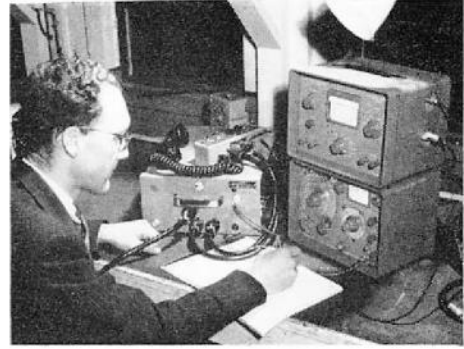
LEFT: For the maintenance of VHF equipment, a wide variety of M.I. test equipment is available. The picture shows Standard Signal Generator TF 144G and F.M./A.M. Signal Generator TF 995A being used in the repair of a mobile unit, one of many employed by a South Wales steel plant. RIGHT: These two instruments, recently introduced by M.I., together provide full facilities for testing mobile transmitter/receiver equipments. John Parkyn, M.I. Design, is using them on the Marconi VHF F.M. Telephone Equipment Type HP 81A
